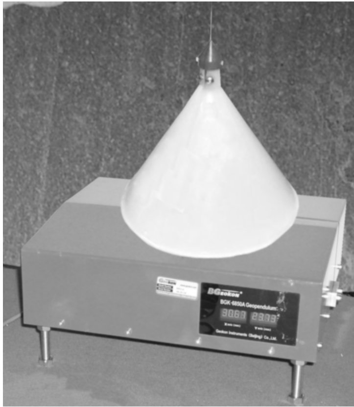
Figure 24 - Conical Drip Shield Installed
