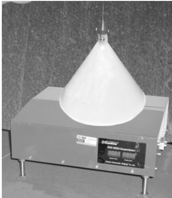
Figure 12 - Conical Drip Shield Installed
