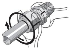
Figure 12 - Tighten Nut Slightly
