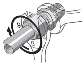
Figure 9 - Tighten One and One-Quarter Turns
