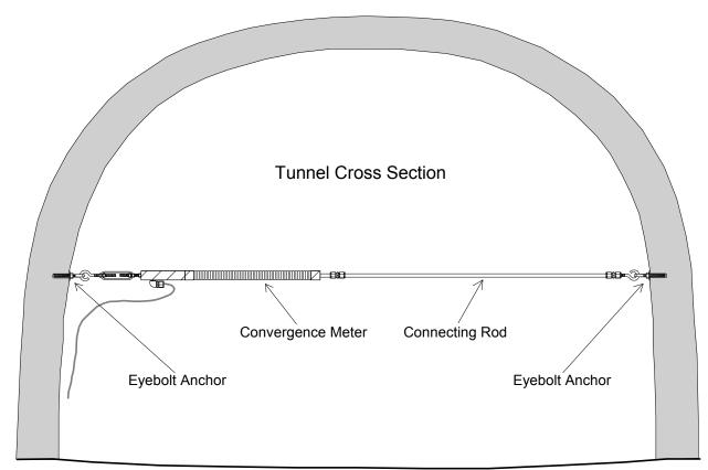
Figure 3 - Model 4425 Convergence Meter Installation
