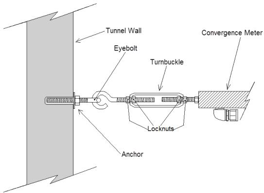
Figure 4 - Convergence Meter Installation Detail - Turnbuckle End
