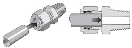
**Figure 7 - Tube Insertion**
