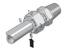
Figure 8 - Make a Mark at Six O'clock
